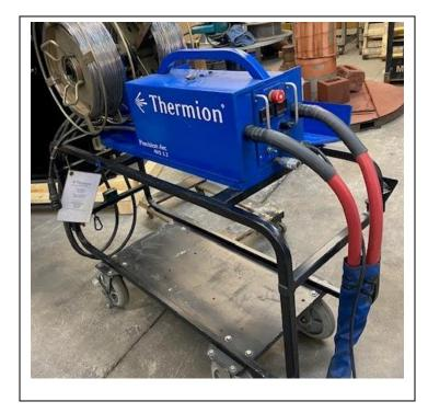
Thermion Precision Arc 3.2 - Fan spray of 1/8" wire - 450-amp power supply.
